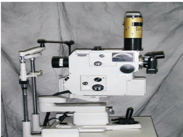
Figure 13.32 Digital spectral retinal oximeter.
