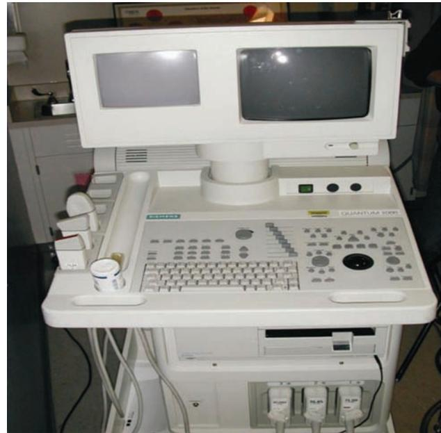
**Figure 13.13** Color Doppler imaging ultrasound machine. (Siemens Quantum 2000, Siemens Ultrasound, Issaquah, WA.)
