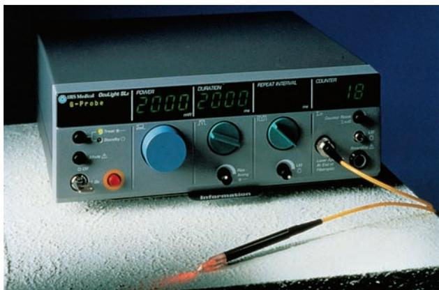
Figure 16.29 The Oculight SLX (Iris Medical, Mountain View, CA) diode photocoagulator.
