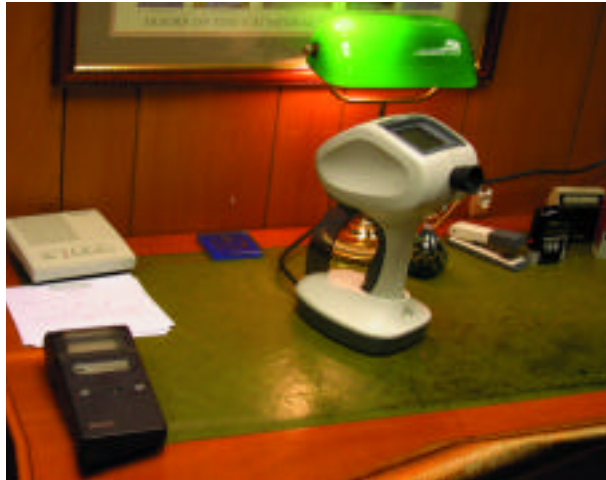
FIGURE 2. The striking point about the PT100 handset is its small size – just 25cm high, 12cm wide and 20cm deep
