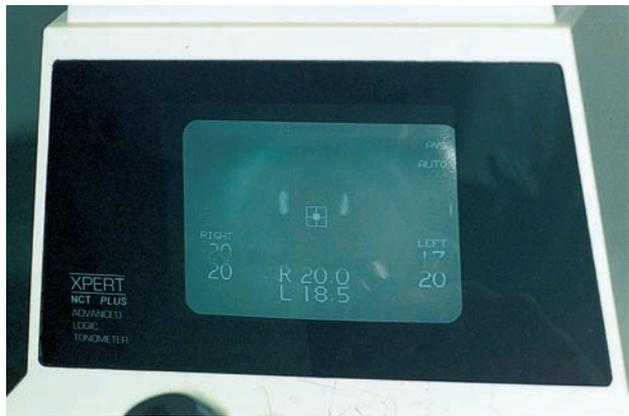
**Figure 4.18** The display of a non-contact tonometer. The eye can be seen faintly in the center of the CRT. The pressure readings obtained for each eye are displayed, with the average in the middle.
