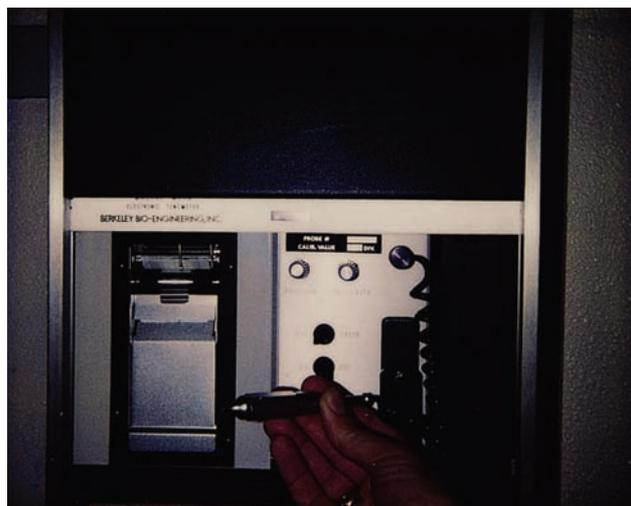
**Figure 4.11 The Mackay–Marg Tonometer.** This is another applanation-type device in which the movement of the tip is sensed by a transducer contained in the hand piece. The bending pressure of the cornea, opposed by the intraocular pressure, is determined. The instrument is useful for measuring the intraocular pressure in scarred, irregular, and/or edematous corneas.
