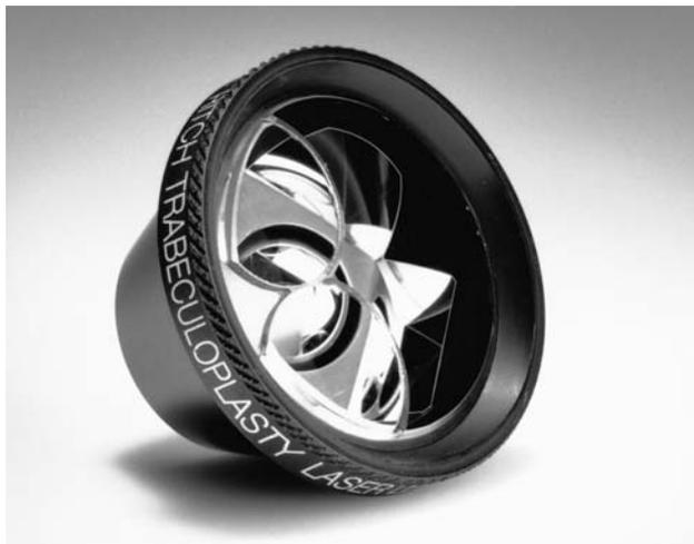
**Figure 16.16 The Ritch lens.** The Ritch lens has two different angles on its mirrors:  $64^\circ$  for the superior angle and  $59^\circ$  for the inferior angle. In addition, a planoconvex button is positioned over each mirror, which provides  $1.4 \times$  magnification. This reduces a  $50 \mu\text{m}$  spot to  $35 \mu\text{m}$  and doubles irradiance. (Courtesy of Ocular Instruments.)
