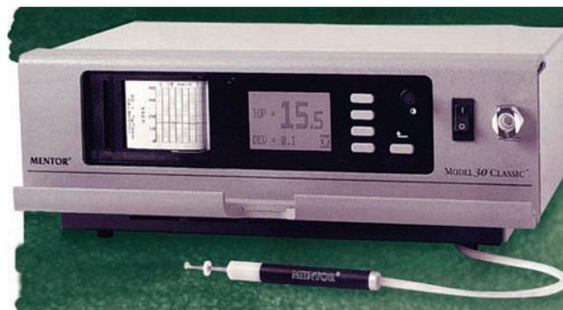
**Figure 4.12 The pneumatic tonometer.** The measuring device consists of a gas-filled chamber with a transducer capable of sensing the pressure in the chamber. As the device is applied to the eye, the counterpressure in the eye pushes back on the tip, raising the pressure on the gas until the end point is reached and recorded, either on a moving paper strip or displayed on a digital readout. This device may also be used for tonography.
