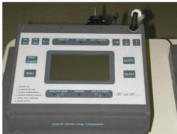
**Figure 13.10** Pulsatile ocular blood flow device. (OBF Labs (UK) Ltd, Malmesbury, Wiltshire, England.)
