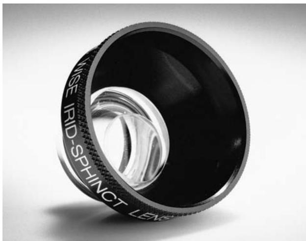
**Figure 16.13 The Wise iridectomy lens.** Using the Wise iridectomy lens as an example, corneal irradiance is decreased 91%, spot size on the iris is decreased 62% (increasing irradiance 7 $\times$ ), and potential fundus irradiance minimized by causing a 230% increase in beam diameter. (Courtesy of Ocular Instruments.)
